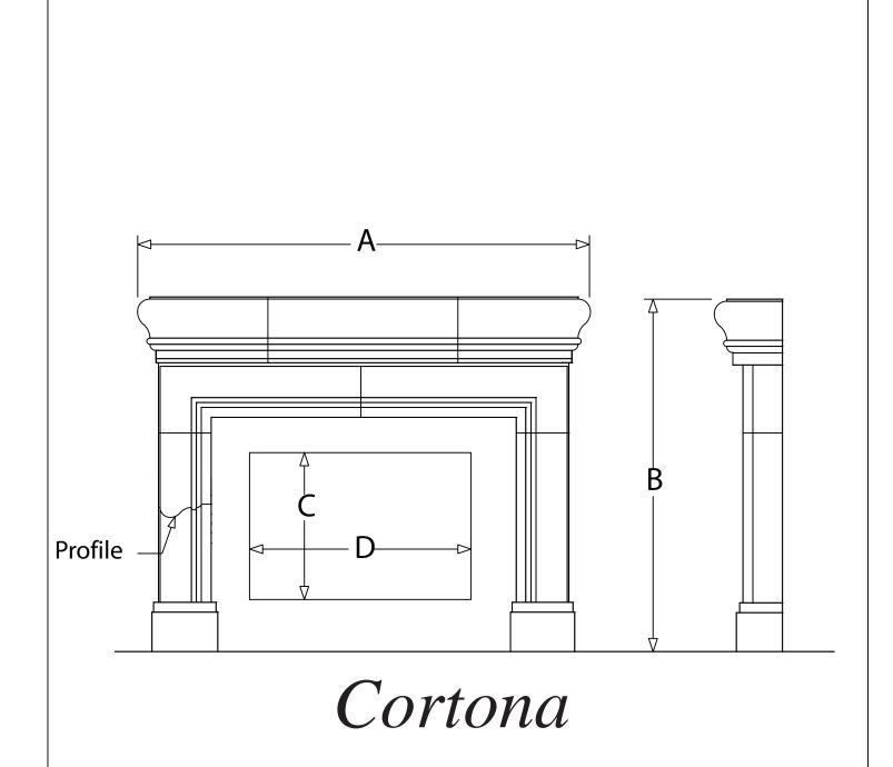
Note: Typical fire boxes are approximately 36" wide (D) and up to 24" tall (C). Please provide AHI with these dimensions so your mantle can be correctly sized. Also, please provide AHI with your desired overall width (A) and height (B)
