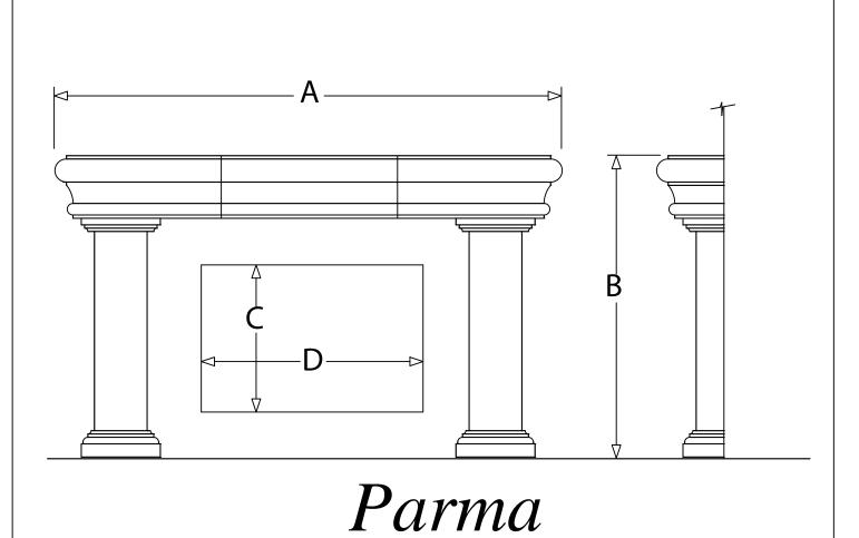
Note: Typical fire boxes are approximately 36" wide (D) and up to 24" tall (C). Please provide AHI with these dimensions so your mantle can be correctly sized. Also, please provide AHI with your desired overall width (A) and height (B)
